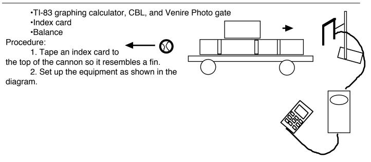
3. The photo gate is arranged so the index card passes through the photo gate. Ideally the card breaks the beam just as the ball exits the cannon. In reality, if the cart's friction is low the photo gate can be set back a bit.
