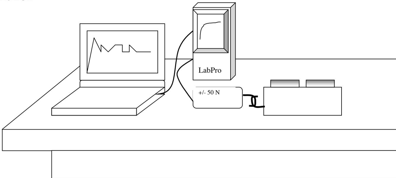
A wooden block is dragged with a Vernier force probe in order to measure the force of friction. The kinetic and static coefficients of friction are determined and it is observed that  $\mu$  does not depend on weight of object and that static friction is greater than kinetic.
